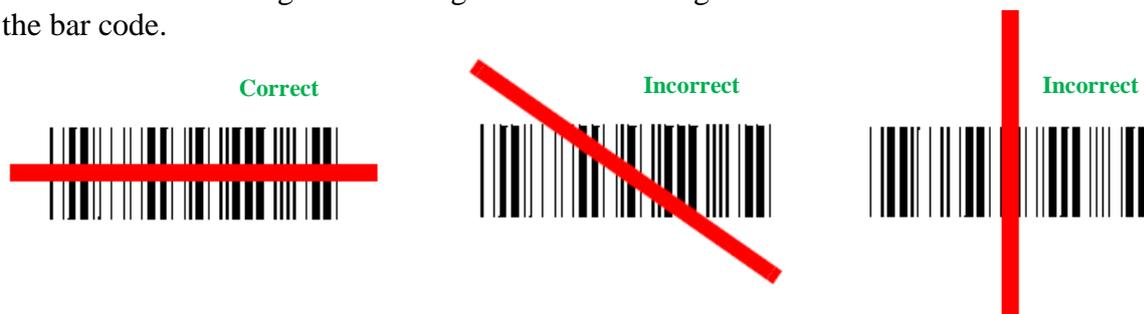
Figure 1: Correct and incorrect scanning
